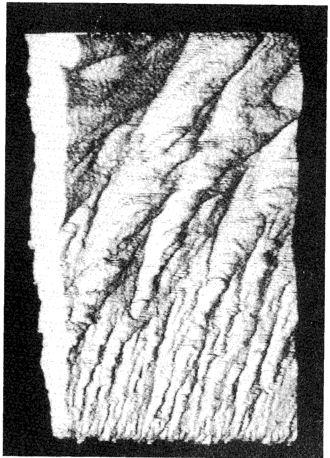
Fig. 2 Volume rendering of 210 images of a rocket motor exhaust jet viewed at 38 and 68 deg off the time axis ( Re = 1.8 \times 10^8 , 140 to 710 jet diam field of view, \sim 2 and 1/3 long time scales displayed).
